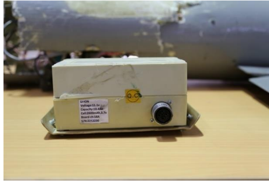
Figure B.38.10 IMG-3053: Li-Ion Battery Unknown Make
