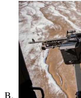
Figure A.58.12 Example of a pintle mount (7.62mm MMG) 45
