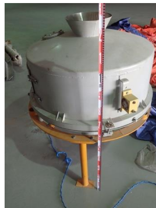
Figure D.36.8 Heating vessel
