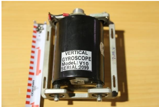
Figure B.38.9 IMG-3047: Vertical Gyroscope V10
