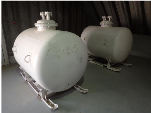
Figure D.36.9 Field storage tanks for liquid bi-propellant oxidiser
