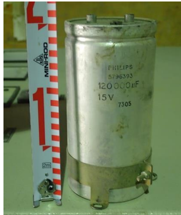
Figure D.36.19 12000UF 15V Capacitor
