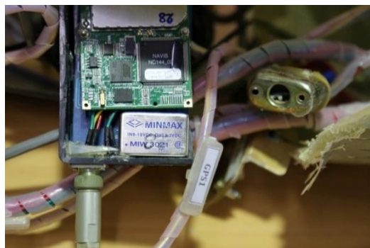
Figure B.38.3 IMG-3029: DC Output Converter MIW 3021
