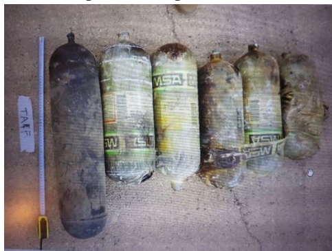
Figure 35.3 MSA composite compressed air bottles
